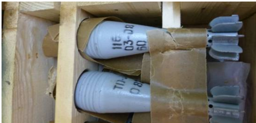
[60-mm mortar rounds manufactured in the Sudan in 2008; 03-08-116: Lot 3, production 2008, factory code: 116 (Sudan)]
